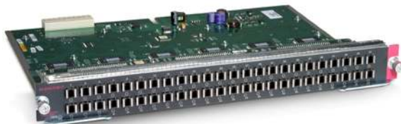
Figure 10. WS-X4148-FE-BD-LC Cisco Catalyst 4500 Series 48-port 100BASE-BX10-D Fast Ethernet Line Card for single strand of SMF
